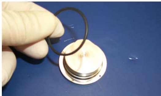
Figure 4-18 Removing the O-ring from Magnetic Pole Piece
