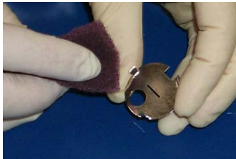
Figure 4-20 Discolored Ground Slit Plate
