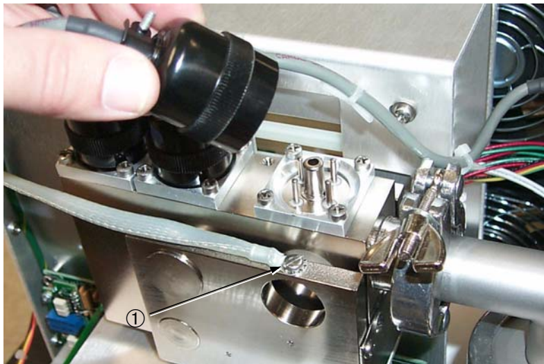
Figure 4-3 Removing the Connectors
