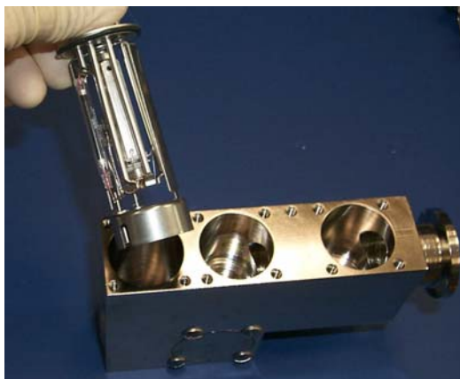
Figure 4-16 Removing the Preampifier
