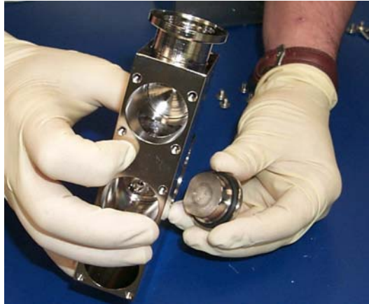
Figure 4-19 Removing the Second Magnetic Pole Piece
