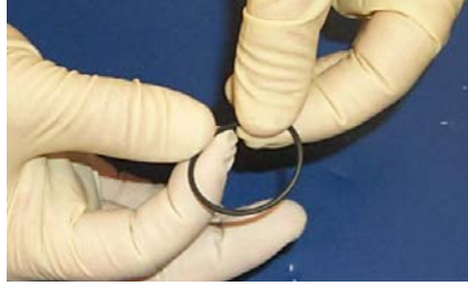
Figure 4-23 Inspecting the O-ring
